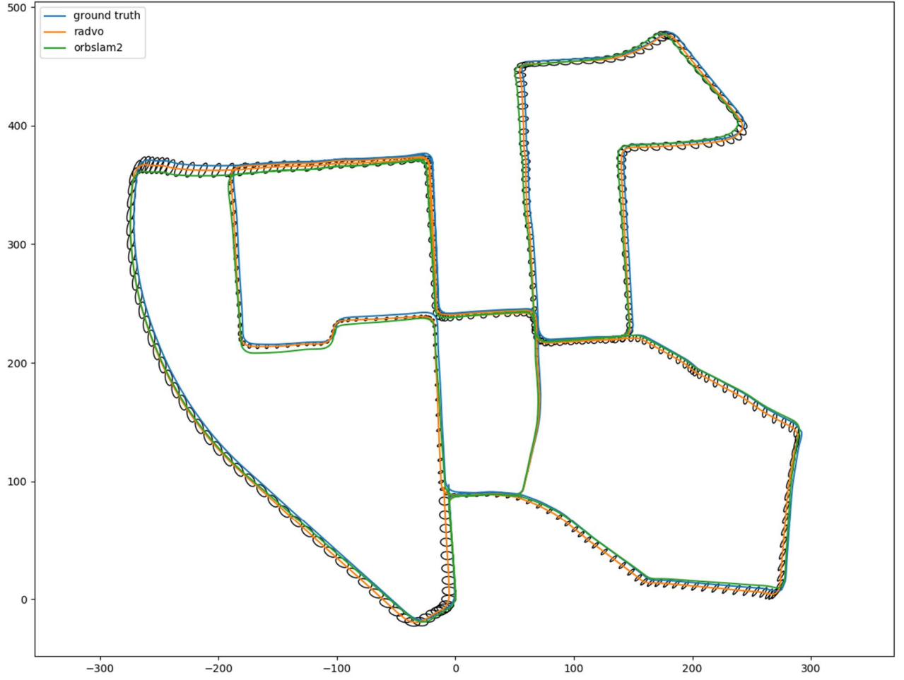
Figure 6: Results on KITTI dataset 00 (orange: ours, blue: ground truth, green : ORB-SLAM2, , black: uncertainty ellipses)
