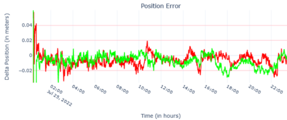
Figure 25: Base Station CEDU : Position Error
